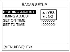
Radar setup menu (heading adjust)
